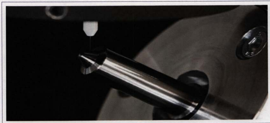
Figure 2 Roughness measurement in the injection hole of an injection nozzle with 50 \mu\text{m} probe.
